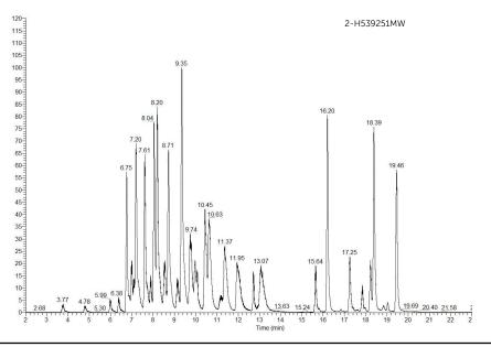
Instrument LC/HRMS – Negative Mode Column/Flow Vanquish C18+ 100 mm x 2.1 mm ID 1.5 um Particle/ 0.2 ml/min
