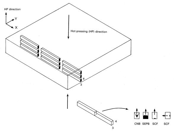
The small arrows show the direction of crack extension.
